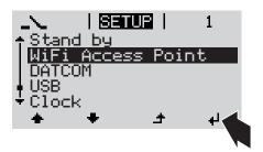
The inverter establishes the WLAN access point. The WLAN access point remains open for 1 hour.
